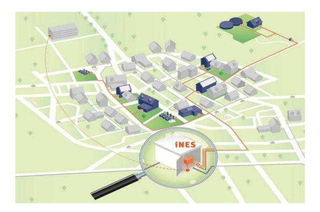
The system's core component is a new and cost-effective control unit (Smart RTU) installed in the distribution substation of the low voltage grid. The control unit communicates with the control sensors and actuators positioned in the grid at only a small number of critical points. Merely 10% to 15% of the network nodes and feed-in stations need actually to be equipped.
